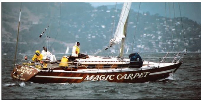
Facing page —At Schooner Creek Boat Works, crew work on the cabintop for the first of two 65' (19.8m) catamarans at left. When it's finished, a second will be infused while the mold is still on the floor. Underneath the hardtop is the mold for the bridge deck. Above —Magic Carpet is a 42' (12.8m) racing yacht built in 1980 in epoxied wood veneer over wood frames. Right —The 70' (21.3m) Rage, also built with wood veneers, has had a successful offshore racing career, including first in class in the 1993 Transpac. Below —Steve Rander, left, founded Schooner Creek in 1977 and sold it to Kevin Flanigan, one of his customers, in 2015, though Rander is still deeply involved.
