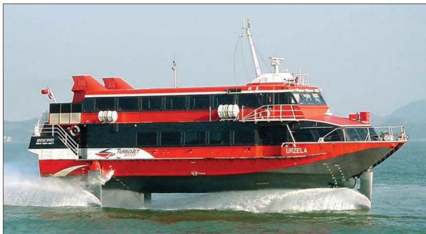
The Jetfoil 929, a hydrofoiling passenger ferry with waterjet propulsion, was also developed by Boeing Marine Systems. Nearly 50 units were built, and most operate in Asian markets.
