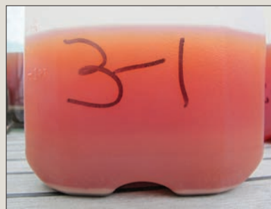
Water-saturated diesel was taken on board in the U.K. Left to right —The three samples represent the water that has settled out at the base of the tank immediately after refueling, 24 hours later (2-1), and then another 24 hours after that (3-1). The rate of water dropout decreased but nevertheless continued for weeks.
