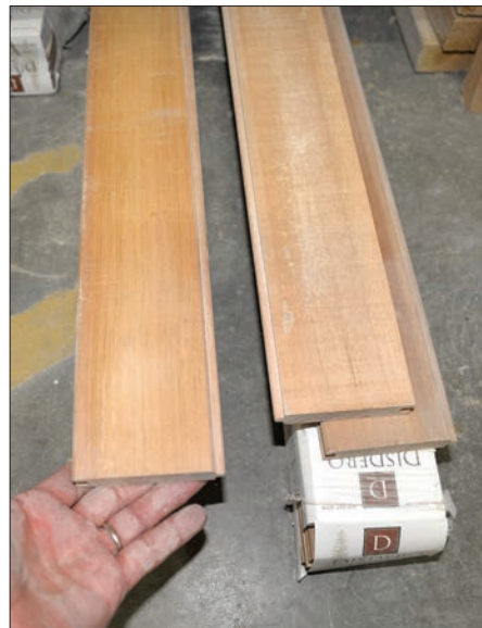
Left —Stations cut in particle board are set up on a strongback. Right —Off-the-shelf cedar tongue-and-groove planks are fastened inside the frames to form a female mold in the shape of the hull.
