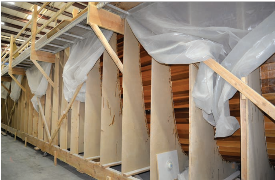
Left —Stations cut in particle board are set up on a strongback. Right —Off-the-shelf cedar tongue-and-groove planks are fastened inside the frames to form a female mold in the shape of the hull.
