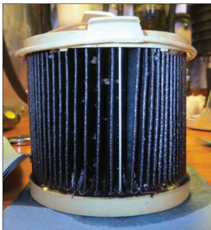
The fouling of this Racor primary filter element is from an ostensibly clean fuel tank treated with a shock dose of Fuel Right. The chemical has broken loose various deposits from within the tank.
