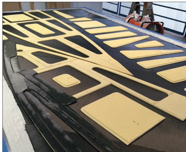
Left —The rigging shop occupies part of the mezzanine overlooking the building's main floor. Right —Full-size patterns are printed on Mylar and then transferred to the material—in this case, Divinycell for parts of the rowboat. CNC cutting was abandoned, as its programming took too long.
