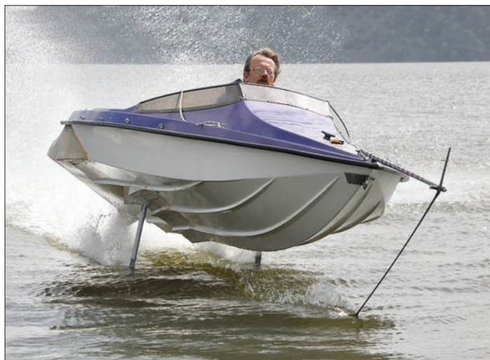
Designer Alexander Sahlin drives an early prototype of the Swedish Foiltwister. It uses mechanically controlled foils, including a wand at the bow to manage foiling height.
