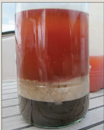
Water-saturated diesel was taken on board in the U.K. Left to right —The three samples represent the water that has settled out at the base of the tank immediately after refueling, 24 hours later (2-1), and then another 24 hours after that (3-1). The rate of water dropout decreased but nevertheless continued for weeks.
