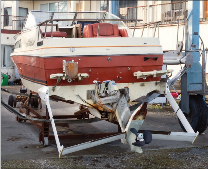
A view of the stern reveals the extension of the outdrive shaft, which keeps the propeller submerged when foiling, and Talaria's anhedral rear foils.
