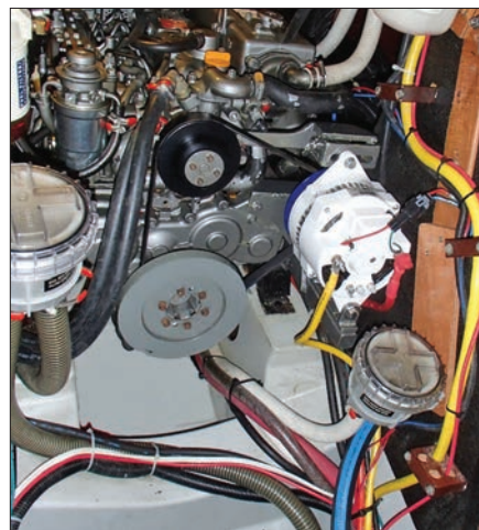
Reverse-mounted alternator with a 10-rib serpentine belt and tensioning device.
