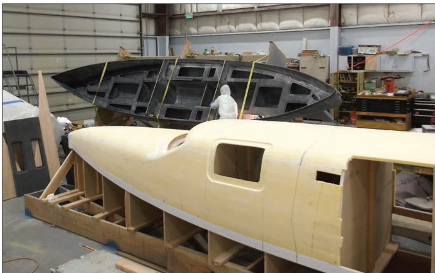
This oceangoing rowboat, commissioned by a U.S. Air Force jet pilot for a planned voyage across the Pacific Ocean, was built by placing foam core over stations. Then, after fairing, carbon fiber cloth was laid over it and wetted out with epoxy resin. Schooner Creek did not make a traditional mold for the boat.
