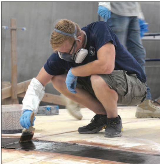
Working on the designer’s specifications to stiffen the structure, project manager Adam Blankinship wets out carbon fiber reinforcements added to the cabintop before the final layer of fiberglass is applied.
