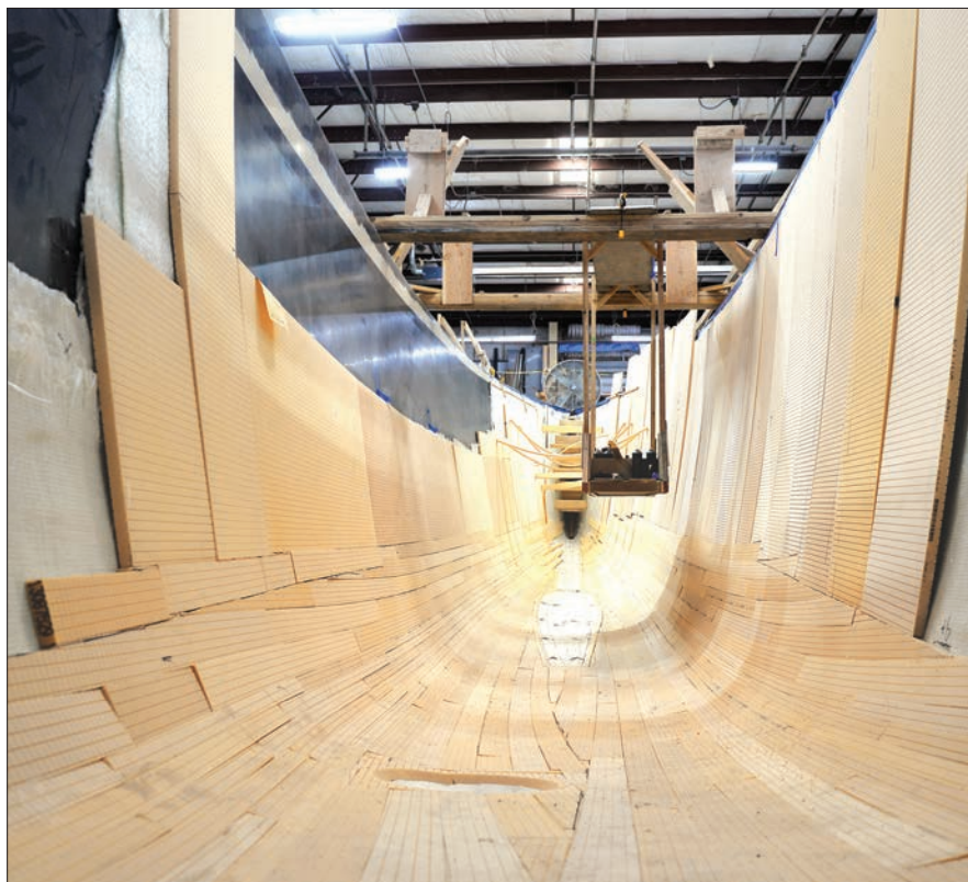
A look inside one of the amas for the second 65’ catamaran shows pieces of Divinycell foam core fitted in place. Densities vary according to location.
