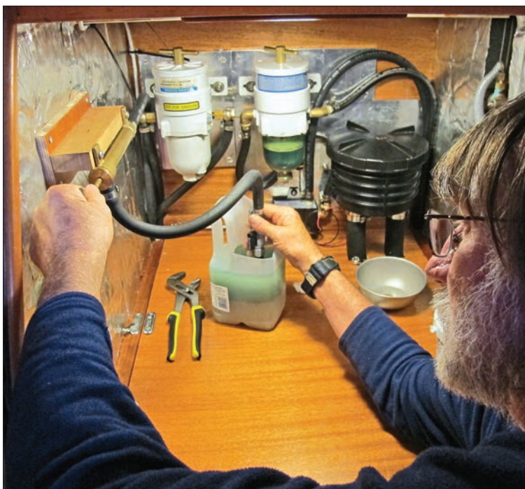
Left —With his manual fuel-tank-sampling pump, the author takes samples at the beginning of every boating season, periodically during the season, and at every refueling. Below —Before any fuel goes in his tanks, the author takes a small sample to see if it is crystal clear.
