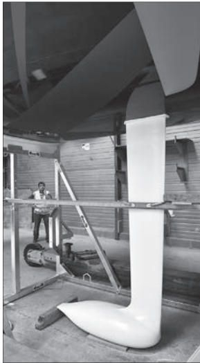
The keel blade and bulb are positioned under the hull, ready for connection.
