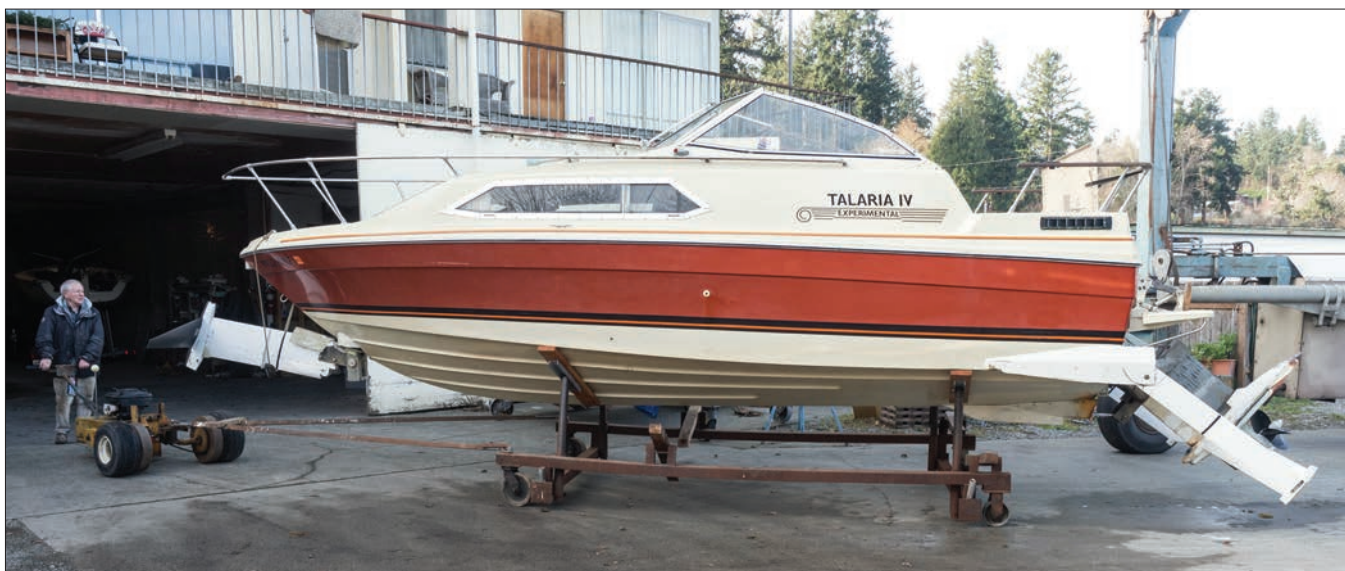
On this vintage yard dolly, the Bayliner with foils is even more odd to behold. But the folding mechanisms Larsen installed enable the boat to fit on a trailer with elevated bunks for road transport.
