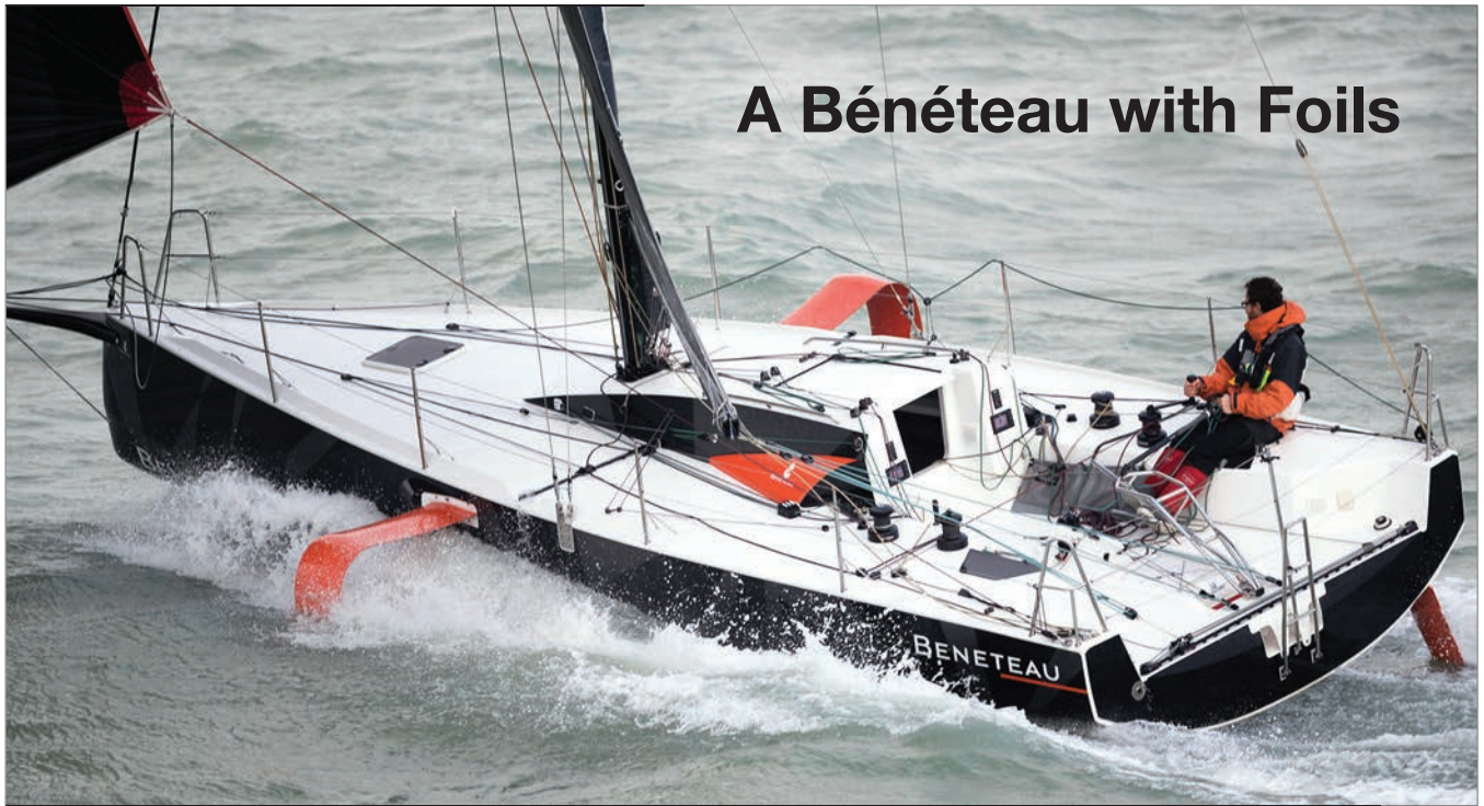
The newest iteration of the one-design composite Figaro Bénéteau 3 is a 32' (9.75m) high-performance sloop with port and starboard curved foils that improve lift and stability. The boat was designed by multihull specialists VPLP Design for La Solitaire URGO Le Figaro, a multi-port race along the French and Spanish coasts.
