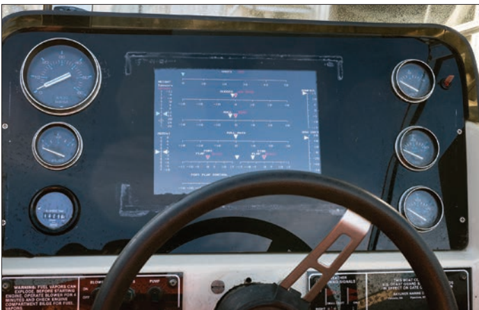
Left —The custom-programmed LCD monitor displays vital data including speed, rudder angle, roll rate, and foiling height.
